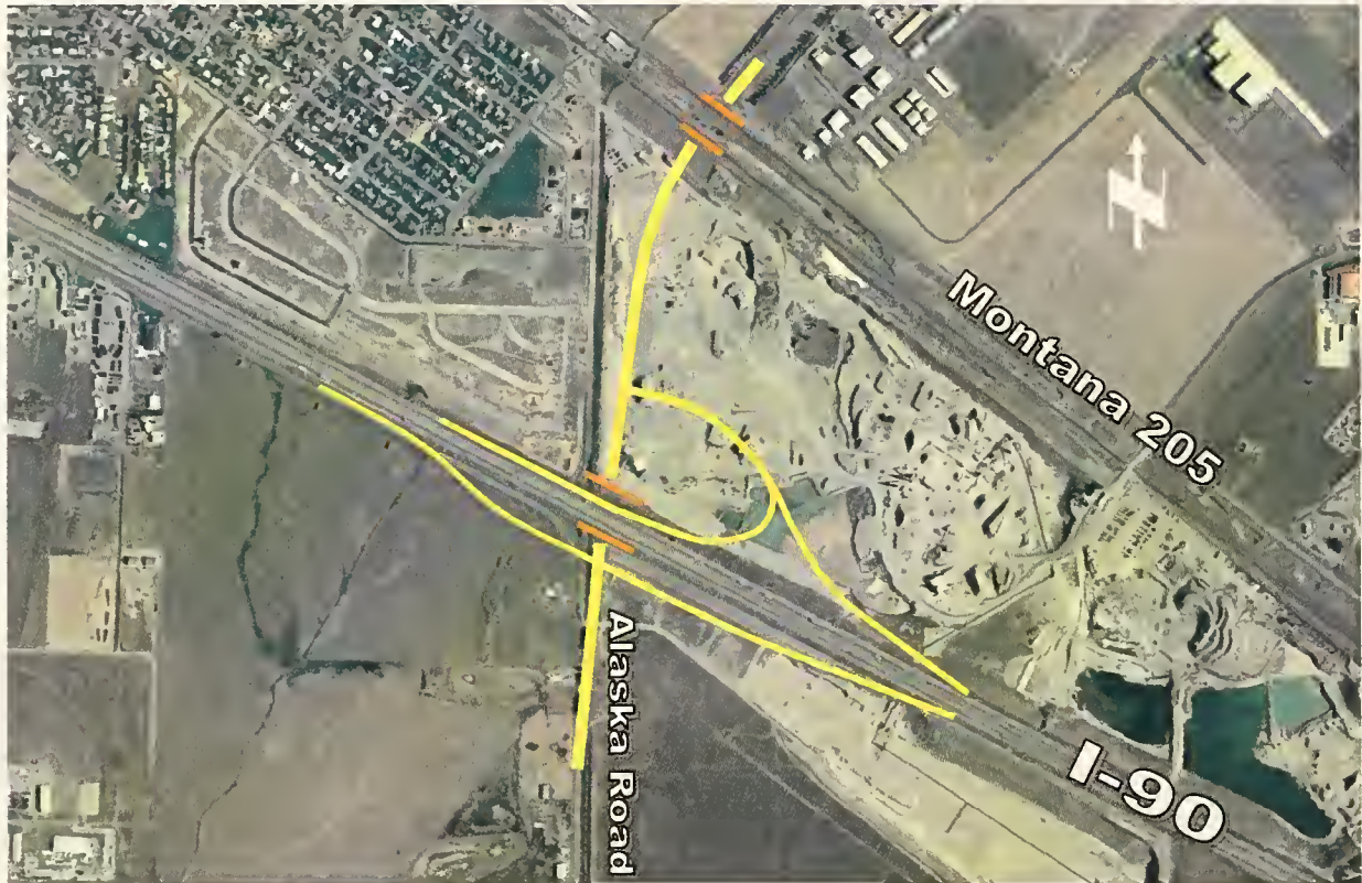
Figure 2-5 Partial Cloverleaf Interchange
